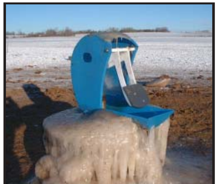
Chipping ice off the pump is the only maintenance required (Photos courtesy Jim Anderson)
