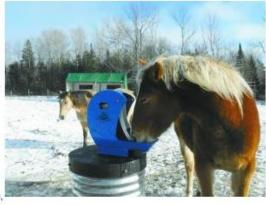
They use geothermal heat to operate without freezing. The animal pushes on a paddle within the drinking hood to reach water that pools at the back of the bowl. As the paddle moves to the back, the pump brings up about one pint of water. Once the animal is finished drinking, the paddle retracts to the forward position, leaving the bowl nearly empty.
