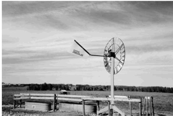
Figure 7. Wind-powered pumping system
