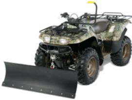
[Broadwood International](#) is now selling the US CycleCountry range of snow ploughs for ATVs and utility vehicles. These are made from a durable steel construction with a 75mm reversible wear strip along the bottom of the plough. Three widths are offered – ATV users can choose between 1.37m or 1.52m, while users of utility vehicles such as Kubota RTVs and Kawasaki Mules get the 1.82m version.
