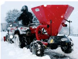
Northern Ireland-based manufacturer **Quad-X** says it now has snowploughs designed to fit most ATVs, plus wider models to suit utility vehicles. Its Supermount mounting system fixes to the underside of the quad and can be used with a number of different Quad-X attachments.
